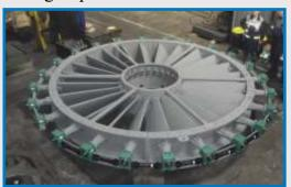
(concerns axial fans) – impeller blade angle adjusted during fan operation through a hydraulic (most applications) or a mechanical actuator.
